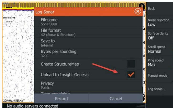
You also have the option to manually initiate an upload to Insight Genesis by going to Files, My Files, Logs, Sonar, choose the log to upload and Select the "Upload to Insight Genesis" button when an internet connection is available.
